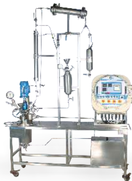
Jacketed reactor with distillation setup & ex-proof electricals
