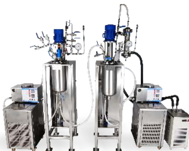
High pressure polytest reactor system
