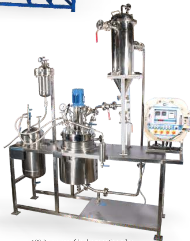
100 ltr ex-proof hydrogenation pilot plant with catalyst charging, catalyst filter with recycle, auto cooling system, vacuum pump & catch pot
