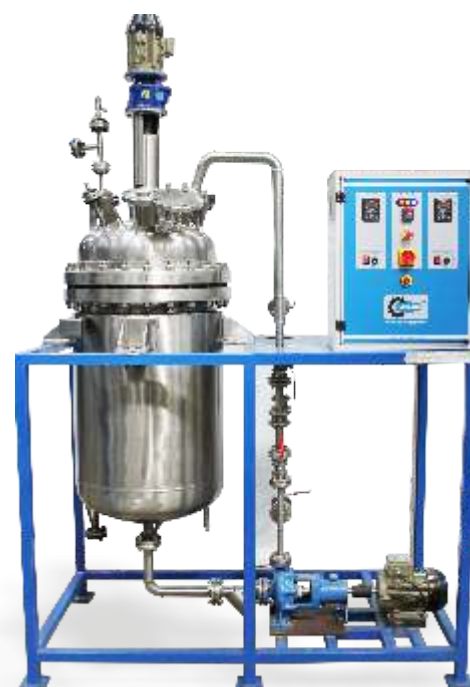
400 ltr Hastelloy reactor with continuous recirculation system
