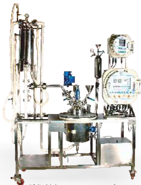
10 ltr high pressure ex-proof system with catalyst filtration & recycling
