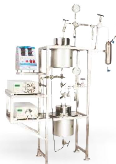
1 ltr extraction vessels in series & parallel for 700 bar pressure with CO 2 pump for extraction of natural products
