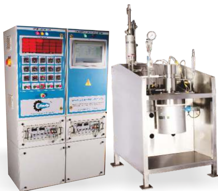
10 ltr autoclave for HPHT corrosion testing
