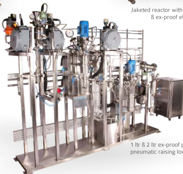
10 ltr high pressure ex-proof system with catalyst filtration & recycling
